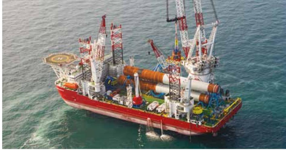
challenges for deck space optimization and crane accessibility which have to be studied carefully and solved in a creative and efficient way.
